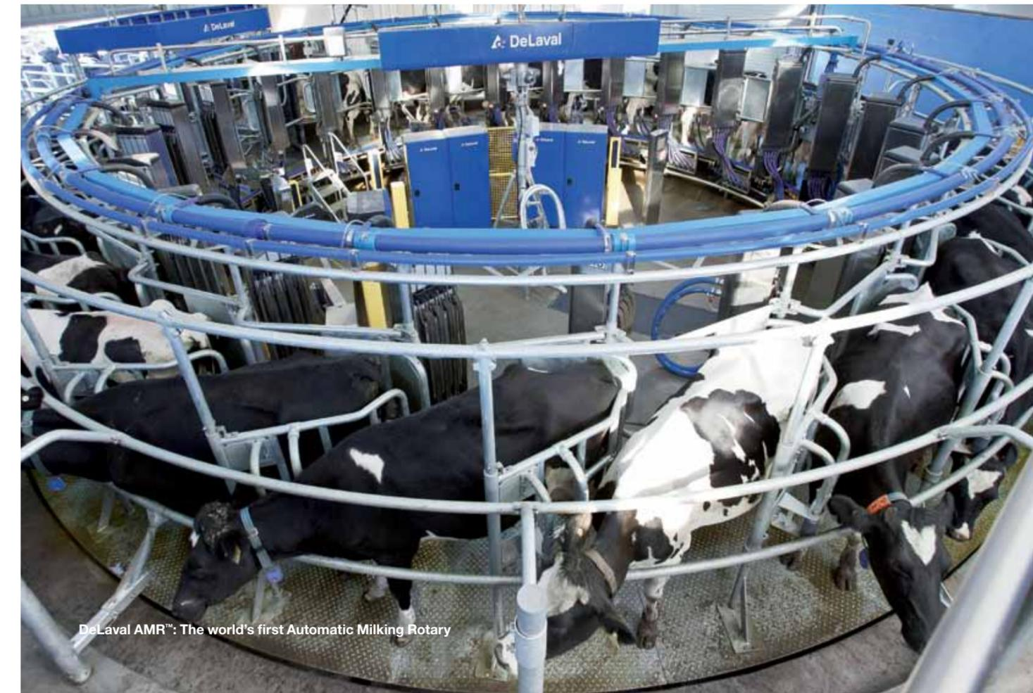
DeLaval AMR™: The world's first Automatic Milking Rotary
